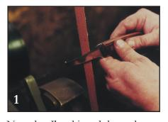
Now that I've thinned down the blade I need to establish the bevel. Photo (2) shows different makes of diamond hones. You want one that fits the hook size of your knife. Work the bevel into the hook (photo 3) and then the blade (photo 4). Some knives are made of a soft enough material that a small rat tail or triangle file can be used. Using files is good for serious roughing in but it produces a serrated edge, which is not desirable. If you start with a diamond hone you may never need a file.
