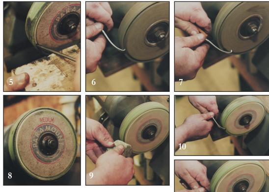
the blade to the wheel. Make sure the edge is down, otherwise your knife may become a permanent fixture in your forehead. Start with the hook **(photo 6)** and sweep through the blade **(photo 7)**, always maintaining the angle of the bevel.
