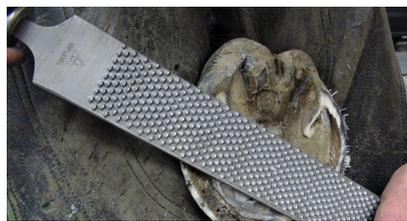
Good aggressive tooth design on the rasp side and a proven file side cut on the Top Level make it one of the more popular styles. Extra width without extra weight helps with efficiency and performance.
