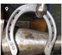
PHOTO 1: Starting on horn, using FootPro rounding hammer.
